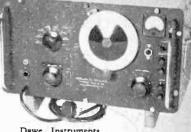
Dawe Instruments Type 802A modulated R.F. oscillator.
