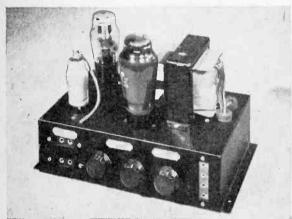
10-watt AUDIO AMPLIFIER. Dimensions  $9\frac{1}{2}'' \times 6\frac{1}{2}''$ . Overall height  $6\frac{1}{2}''$ . Two Channel Input. Tone Control. Heavy duty Output Transformer matched to 3, 8 and 15 ohms. Valves EF36, 5Z4, KT66. Intended for the record enthusiast. Highest possible efficiency, overall gain, stability and equality of reproduction. Eminently suitable for Concert Work, booster amplifier, standby fer amateur transmitters, paging system, etc. Amazing value. Price £8.8.0
