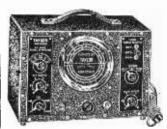
TAYLOR ALL-WAVE SIGNAL GEN-ERATOR. Model 65B. 100 Kc/s to 46 Mc/s. 6 scales. A.C. Mains-operated. Price £15,10.0.
